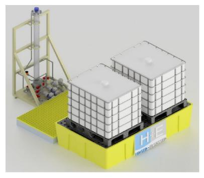
When your rate of chemical consumption is too high to use 25 litre drums but too small to consider bulk tanker deliveries, purchasing chemicals in 1m³ Intermediate Bulk Containers (IBCs) can be a good and economic choice. H+E's IBC Chemical Dosing systems are pre-assembled prior to delivery and connect directly to the liquid outlet of the IBCs.
