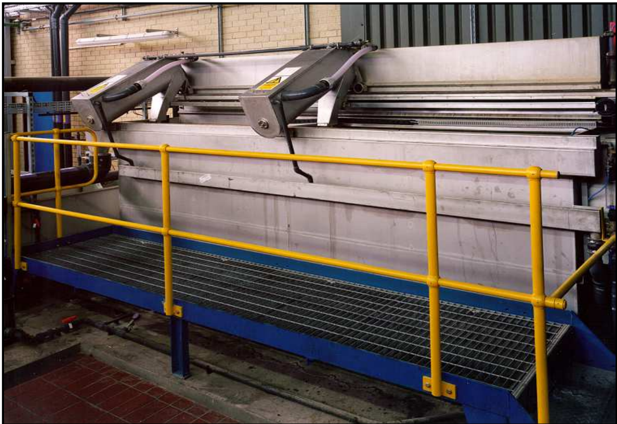
TOVEKO filter installed at Continental. The platform along the front allows convenient access for operators
