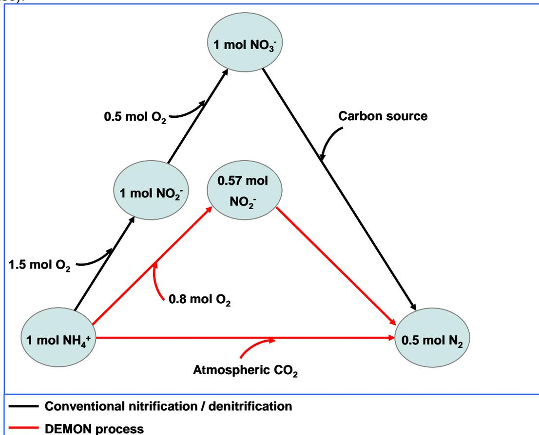
**DEMON® process versus nitrification and denitrification: Energy balance**
