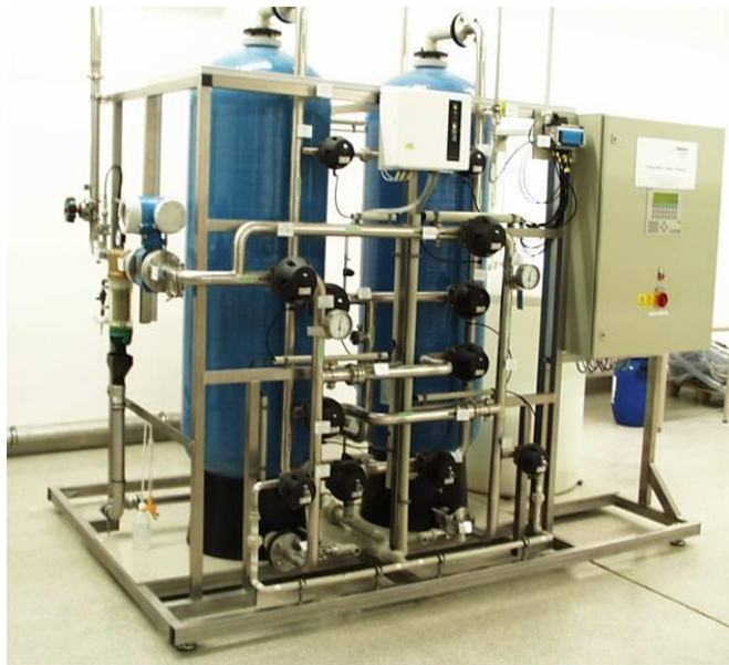
Typical small Ion Exchange system for Rinse Water Recycling
