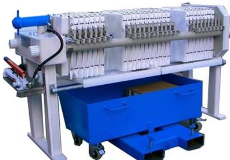
Typical small filter press for sludge dewatering
