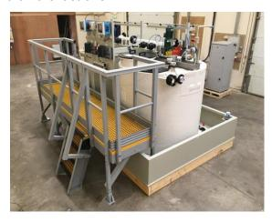
What you can see here is a pre-assembly complete with tanks, bund, access platform, mixers, instruments, chemical dosing system etc., all pre-wired and tested in our factory. If you have a requirement, whether for a one-off fabrication, a series of parts, or a complete factory-built and tested system, please tell us exactly what you need and we will be pleased to discuss those needs with you.
